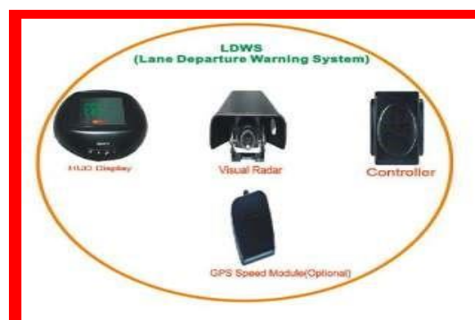
Figure 6: The Lane Departure Warning System
