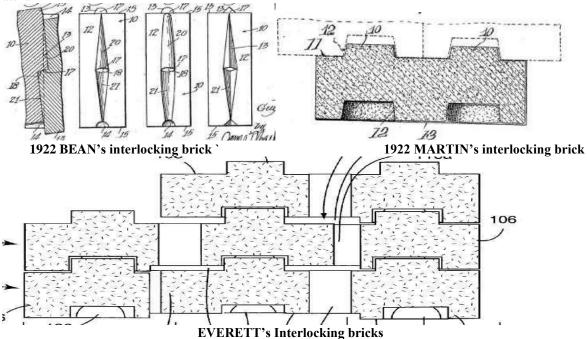
Similarly, patent based on interlocking in this field US. Patent. Nos. 5379565 (Fabien Vienne), 2185497 (Cilento), 4314431 (Rabassa), 2145404 (Mueller), 1984393 (P.brown) are available . but for ideal and perfect interlocking brick, A number of requirements for systems of this type are as follows:
